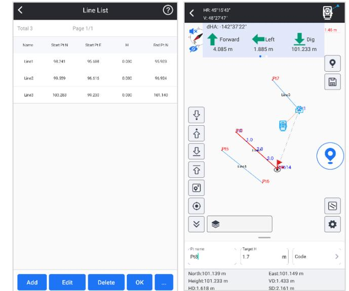
User is allowed to manually choose points from library, line will be formed by program automatically. Then user input interval distance, setout points will be calculated out and displayed on screen.
