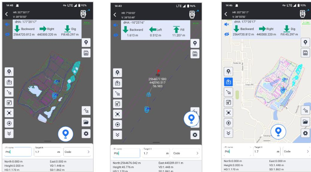
CAD Stakeout allows you to import **CAD basemap** and stakeout it, without inputting point coordinates one by one.
